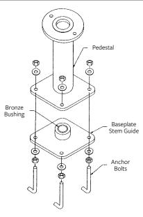
FIGURE 5 - 19 BASE PLATE STEM GUIDE
