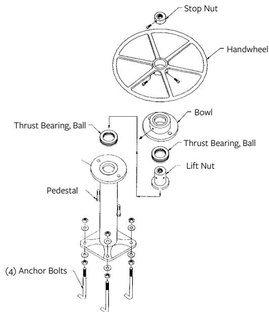
H1B OR H2B - LIFT MOUNTED ON PEDESTAL
